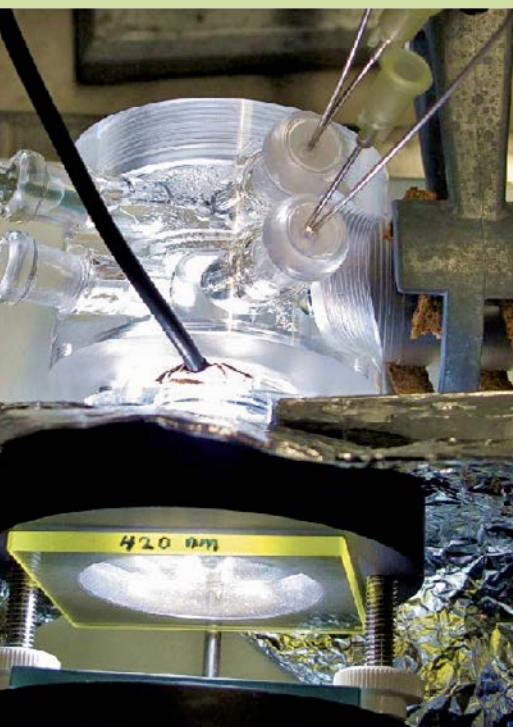
Figure 1: In a home-made photoelectrochemical cell the splitting of water into hydrogen and oxygen occurs under visible light irradiation (wavelength > 420 nm) using a newly developed hybrid photoelectrode.
