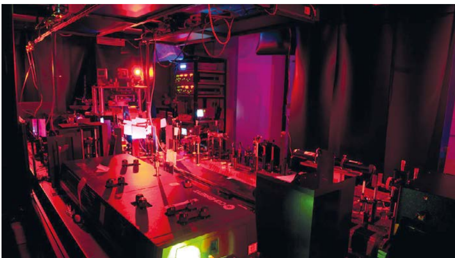
The laser setup for ultra-fast Kerr-Rotation spectroscopy on wide-bandgap semiconductors. Photo by Jens Sundheim.
