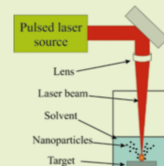
Figure 1: Schematic view of the generation of nanoparticles by laser ablation
