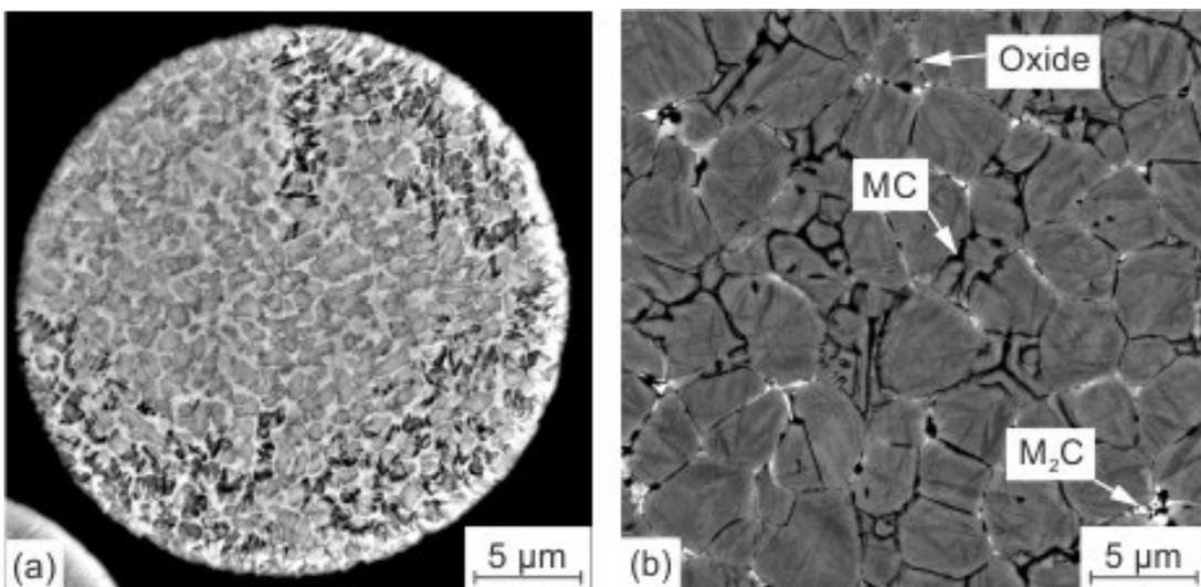
Figure 2: Characteristic microstructural solidification structures of the PM HS 3-3-4 powder droplets.
