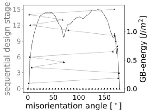
Figure 2: Sampling the energies a symmetrical tilt grain boundaries.
