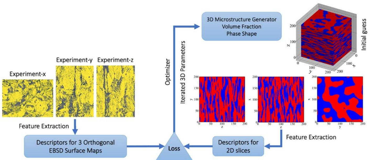
Figure 1. Representation of workflow to reconstruct 3D microstructures from surface maps.
