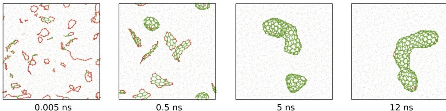
Figure 1. Nucleation and growth of fullerenes in an argon atmosphere.
