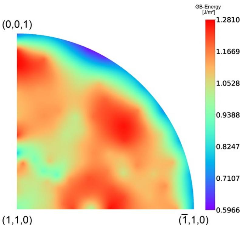
Figure 3: Fundamental zone of grain boundary energies of a low angle grain boundary with different boundary plane inclinations.
