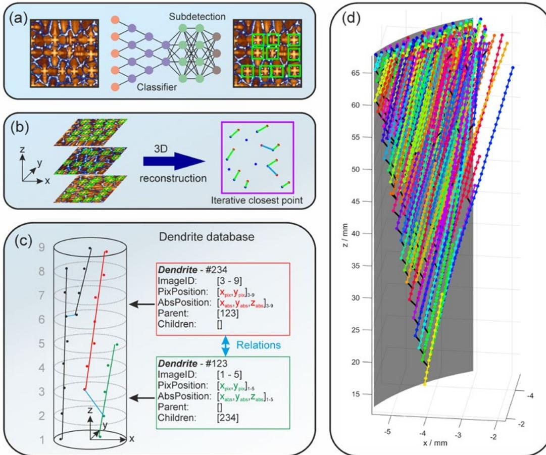
Figure 1: Architecture of a deep-learning assisted automatic 3D dendrite characterization method.
