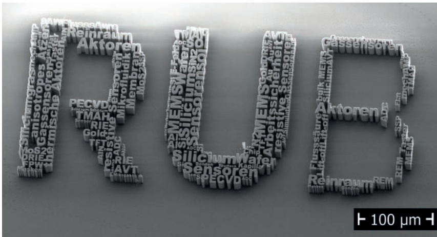
Figure 1: Micro sized RUB word cloud made from silicon via DRIE.
